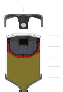
Activation cap with integrated gas generator (PA GF)
